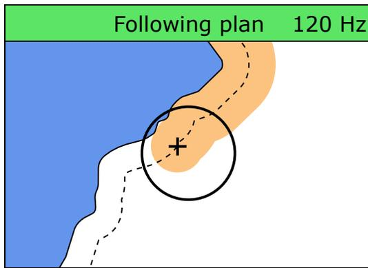
**Figure 6: User interface:** This display shows the shapes of the plan (blue polygons); the path that the tool is actually following, which is those shapes offset by the tool's radius (dotted line); the tool's current position (cross); the area cut by the tool (shaded area); and the range of the tool's position correction (black circle). As long as the user keeps the tool path within the correction range, the tool should be able to follow the plan.
