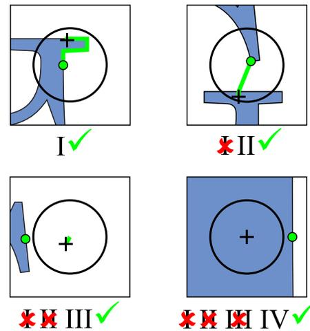
**Figure 5: Freeform motion paths:** Each box illustrates a case in which a different path (described below) is used, due to the higher-preference paths being infeasible. In each box, the cross is the current position of the tool, the circle is the range of the positioning system, the green dot is the target position, and the green path is the selected path.
