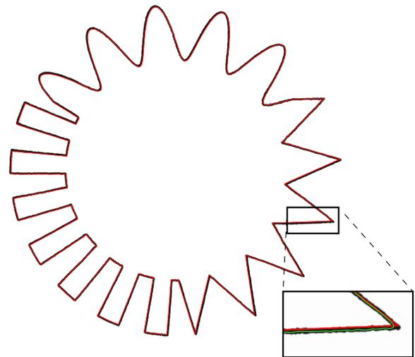
**Figure 10: Accuracy:** A scan of a plotted pattern (6" wide) shown with the design that was used to create it (red). The inset shows an expansion of the area of worst error, with the addition of the line fit to the scan for analysis (green). Note that even here the error is only on the order of the width of the pen.
